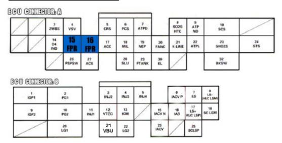
These wires are meant to be tapped into the wires on your stock OBD2b ECU Plugs.
